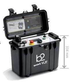
**MWT:** the recently introduced **Monitored Withstand Test (MWT)**, a combination of Withstand Testing and Tan Delta Diagnostics in compliance with IEEE 400.2-2013, can be performed.
