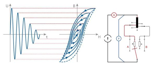
Figure 1: Demagnetizing the transformer core with sinusoidal signal
