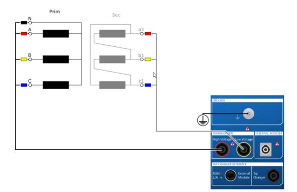
Figure 2: Typical connection set-up for a Star-Delta transformer using TESTRANO 600
