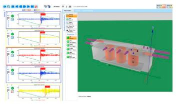
Figure 9 Acoustic signals of piezo sensors
