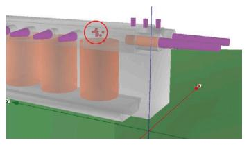
Figure 10 Location of PD at the high-voltage exit of phase 1U
